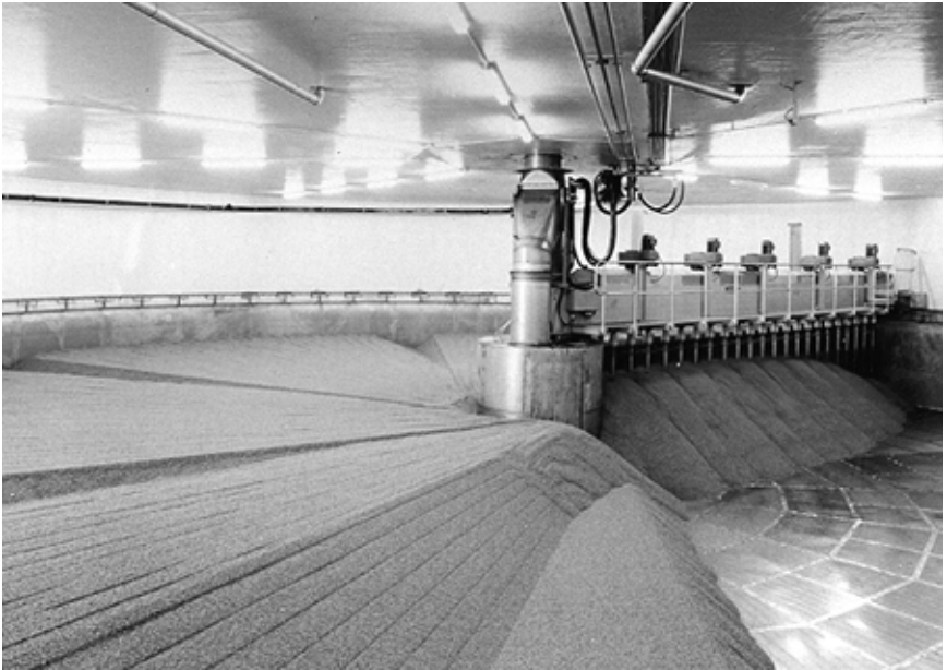
Fig. 9.7 Fixed floor germinating vessel – loading in progress (photograph courtesy of Seeger GmbH).
