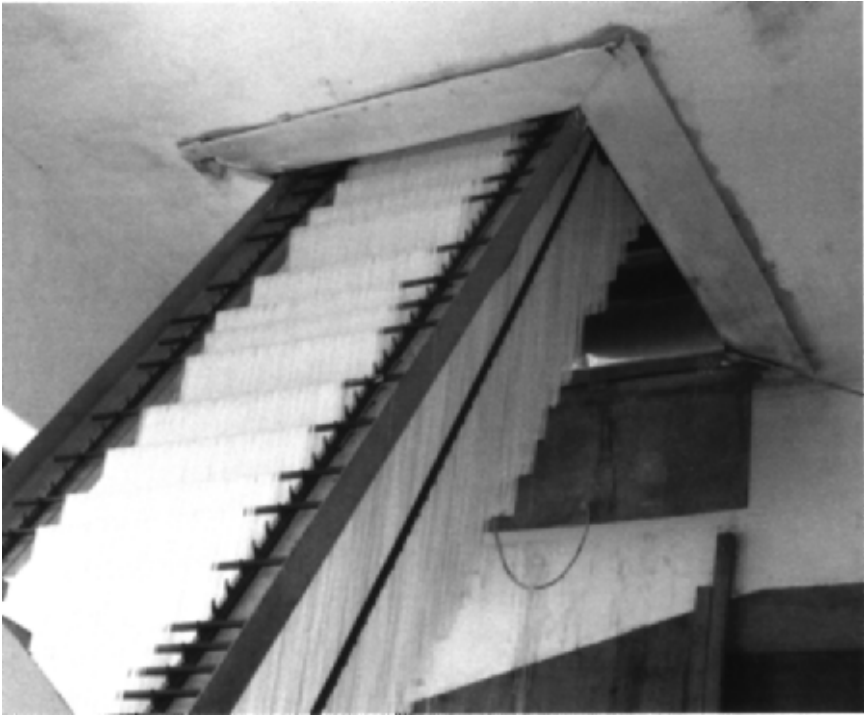
Fig. 7.6 Commercial noodle manufacturer's continuous removal of white salted noodles from temperature and humidity controlled drying areas.
