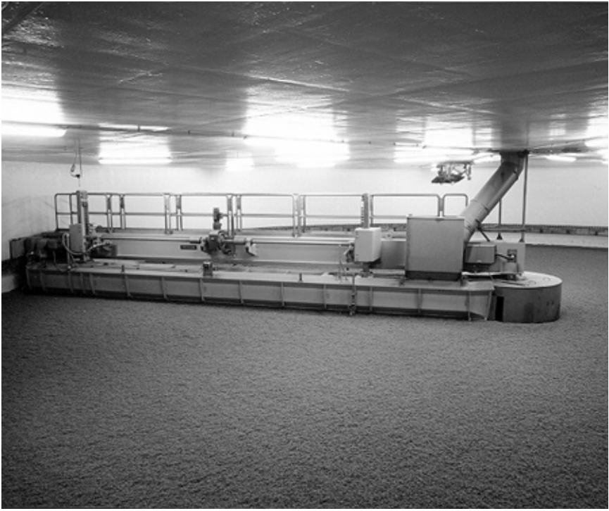
Fig. 9.8 Fixed floor kilning vessel – fully loaded (photograph courtesy of Seeger GmbH).
