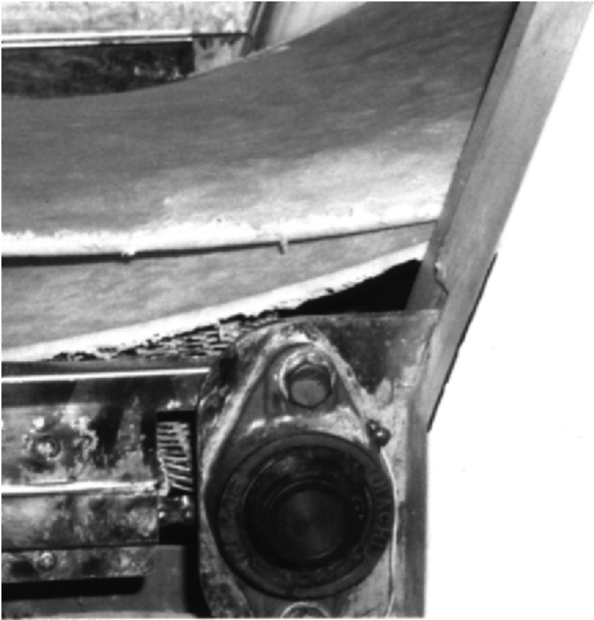
Fig. 7.7 Lamination step in alkaline noodle production using compound rollers.
