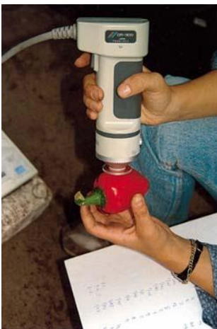
Fig. Objective colour measurement with a colourimeter
