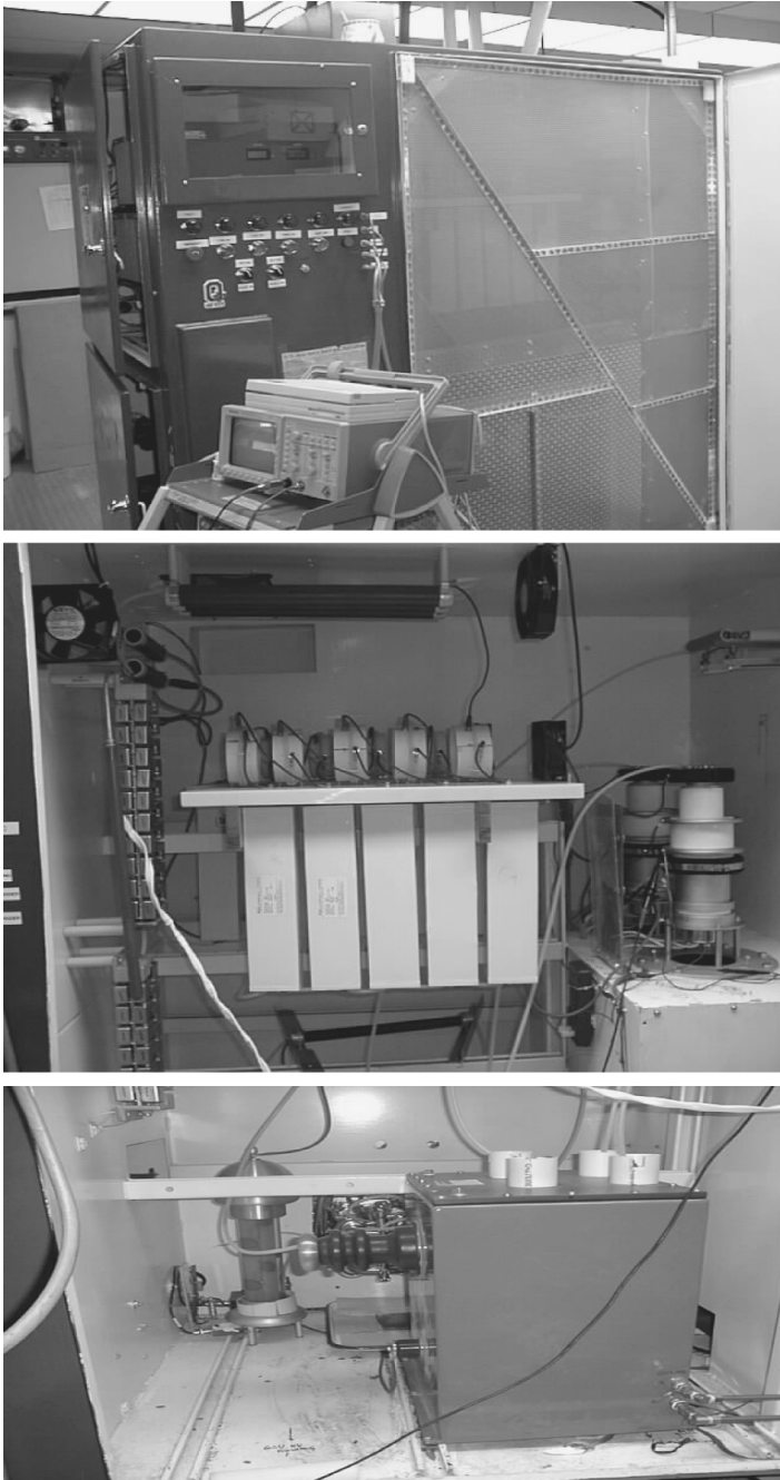
FIGURE 14.2 Pilot plant PEF generator (OSU-2C): bipolar, 50 kV/20 kW.
