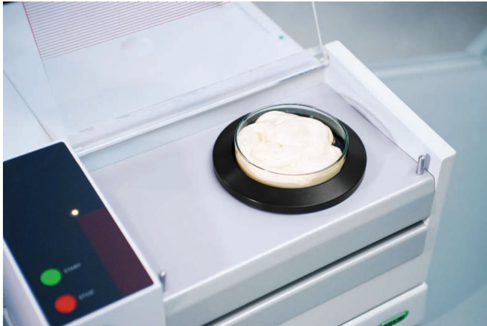
Plate 9 NIR measurement by reflection through the bottom of a Petri dish (printed with kind permission of Büchi Labortechnik, Essen, Germany).
