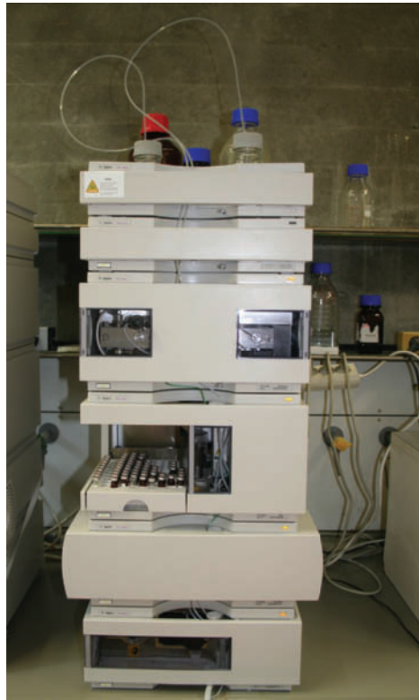
Plate 13 HPLC with (from top to bottom) eluent containers, degassing unit, high pressure pumps, sample vials and injection unit, column chamber, detector (photo: G. Merkh, University of Hohenheim).
