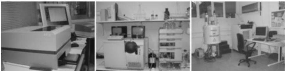
Fig. 4.3 Advanced instruments used for laboratory quality control – ELISA reader, HPLC-MS/MS and NMR spectrometer (from left to right).
