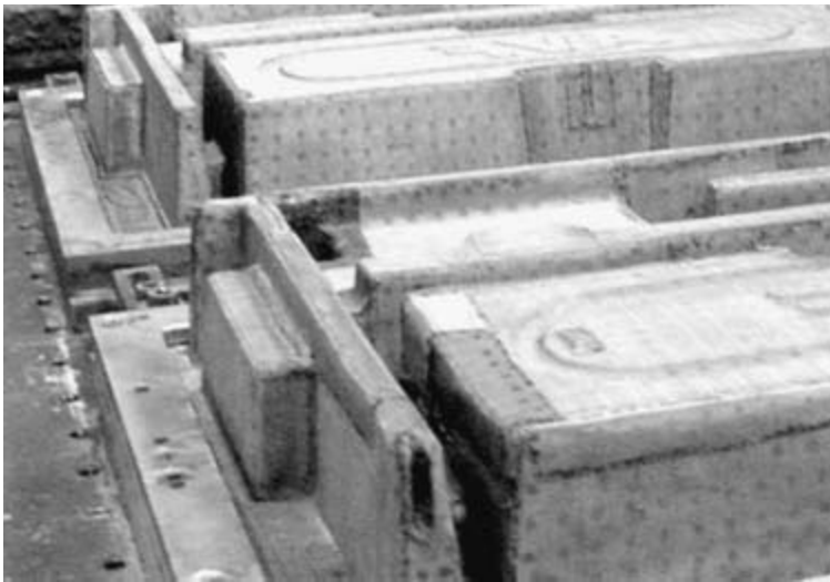
Figure 14.9 Gauze used to mesh the mould tool surface.
