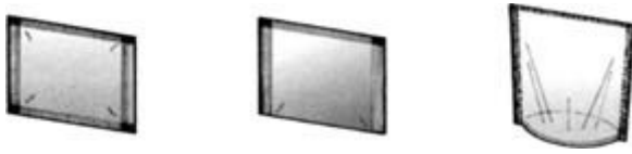
Figure 3.18 Typical horizontally formed pouches/sachets with 3-side sealing, 4-side sealing and base gusset providing a 'stand-up' feature. (Reproduced, with permission, from Rovema Verpackungsmaschinen GmbH.)
