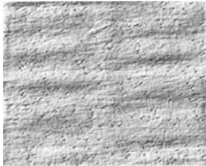
Figure 11.56 Wash-boarding effect of print on corrugated board surface with low grammage white top double face.
