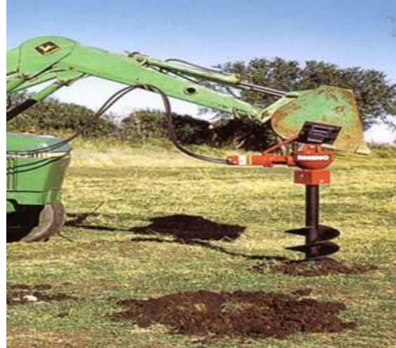
Tractor operated Post hole digger- hydraulic drive
