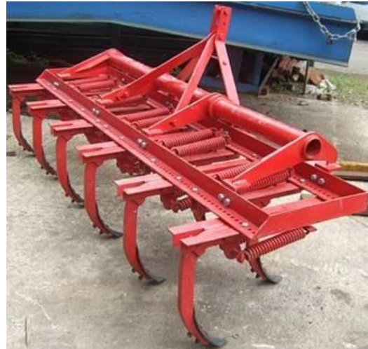
Tractor drawn cultivator- spring loaded tines
