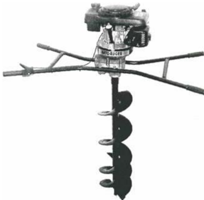
Engine operated post hole digger - manual handling
