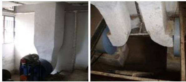
Fig. 11.24 The blowers fitted near the pasteurization chambers for circulation of fresh air and steam
