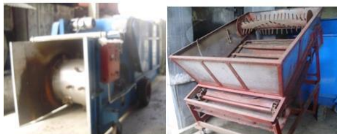
Fig. Turning machines fitted with rotators for turning of composts and filling inside the tunnel.
