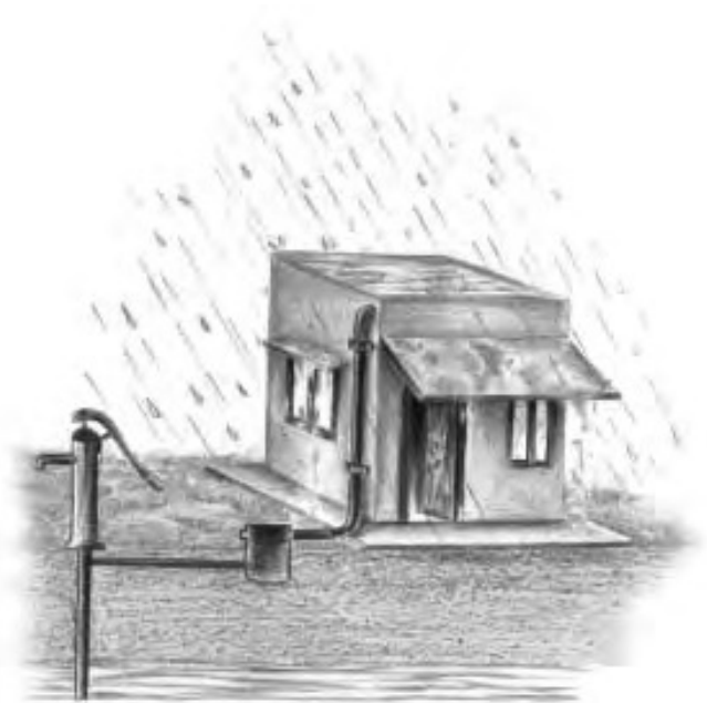
(a) Recharge through Hand Pump
