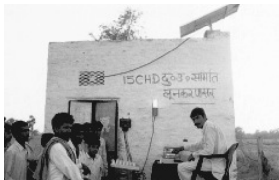
Fig. 5.12: Solar operated electronic milk testing equipment
