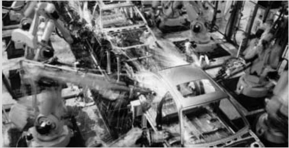
Figure 14.6 : Robot welding the car body
