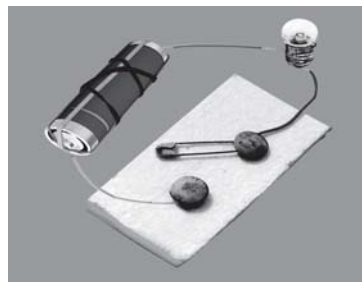
Fig 12.9 An electric circuit with a switch
