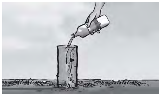
Fig. 9.5 Measuring rate of percolation
