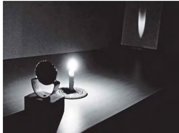
Fig. 15.15 Real images formed by a concave mirror
