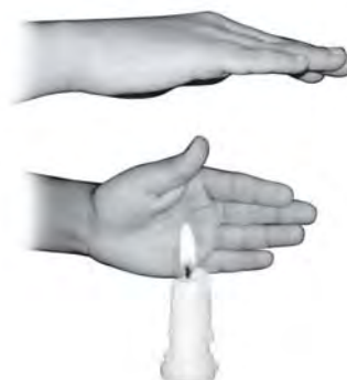
Fig. 4.10 Transfer of heat by convection in air
