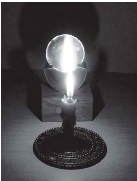
Fig. 15.16 Virtual image formed by a concave mirror
