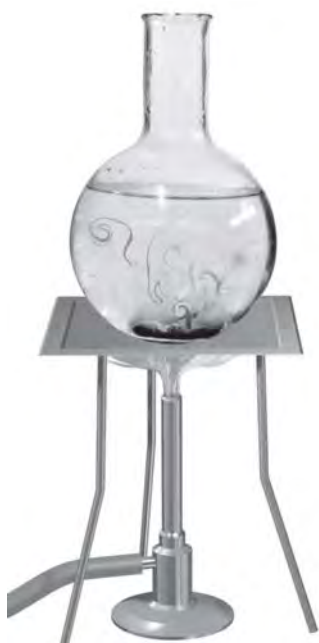
Fig. 4.9 Convection of heat in water
