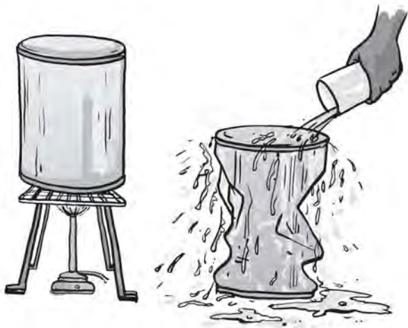
Fig. 8.2 Can with hot water being cooled
