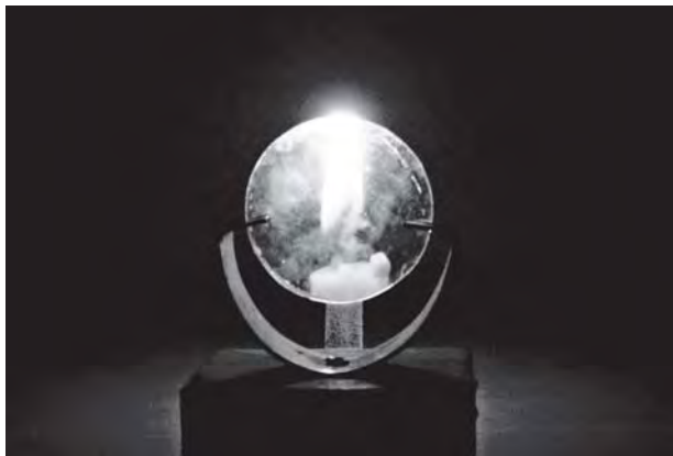
Fig. 15.26 Virtual image formed by the convex lens
