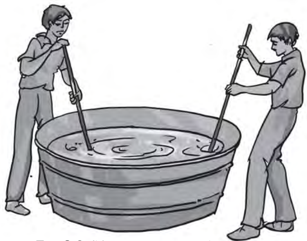
Fig. 3.8 (b) Scouring in tanks
