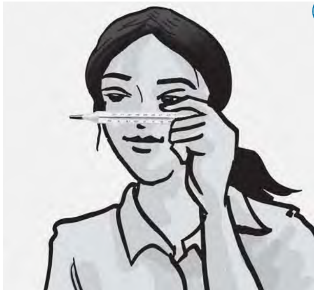
Fig. 4.3 Correct method of reading a clinical thermometer
