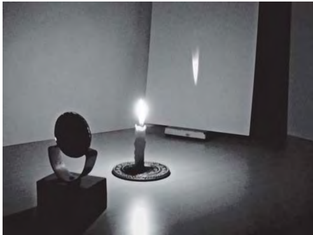
Fig. 15.15 Real images formed by a concave mirror
