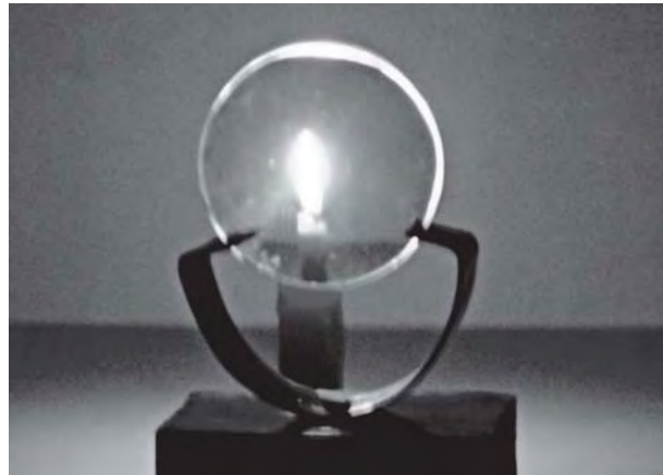
Fig. 15.27 Image formed by a concave lens
