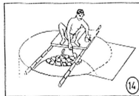
Closing of dome with bricks
