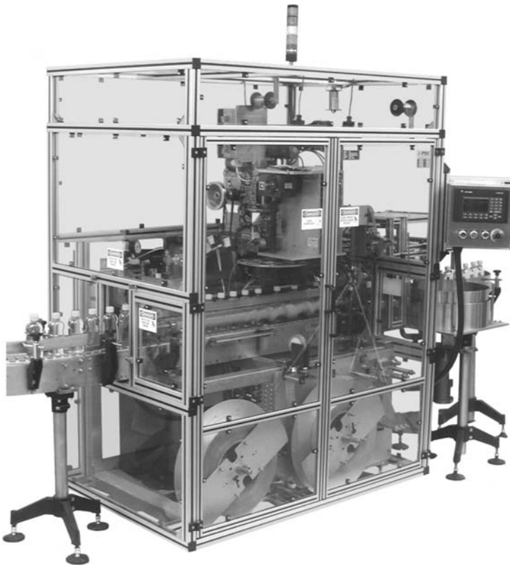
FIGURE 19.8 Example of machinery applying a tamper-evident band (Source: PDC International Corporation).
